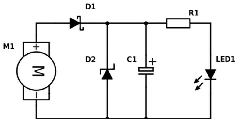
The circuit diagram for the Windup Torch is shown above. It is a very simple circuit. The motor (M1), acting as a generator, powers the circuit when turning the handle. The faster rotation of the generator the higher the voltage supplied to the circuit
