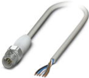
Sensor/Actuator cable, 5-position, PP-EPDM halogen-free, Gray RAL 7035, Plug straight M12, A-coded, on Free cable end, Cable length: 3 m, Hygienic design, With high-grade steel knurl
