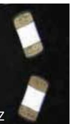
0402 product line extension of Z type plating (Sn over Ni) in the C04 (0402) case size with its Ultra-Low ESR UL dielectric material. Previously the C04 product line was only available in "S" type plating (Au flash over Ni).
