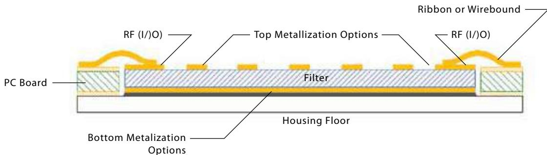
The above illustration demonstrates the mounting of a typical chip and wire filter. The circuit is relieved to accommodate the filter. The bottom surface of the part is attached directly to the system ground plane using conductive epoxy. Wire or ribbon bonds are launched from the circuit to the filter I/O pad. In a typical application a channelized housing would sit over the filter to provide adequate RF shielding.
