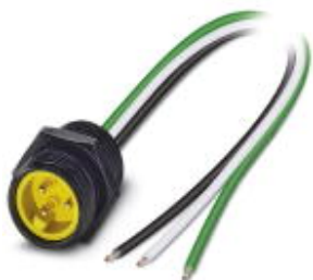
Flush-type connector, 3-position, Plug, straight, 7/8"-16UNF, on free cable end, Front mounting, with 1/2 inch-14 NPT mounting thread, Individual wires, cable length: 1 m
